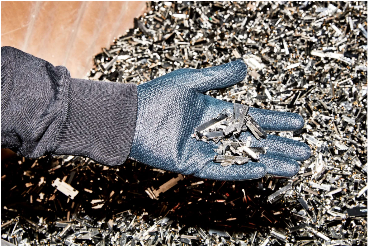
Disassembled iPhone Taptic engines containing rare earth metals, tungsten, copper, steel and gold © Valentina Vos
